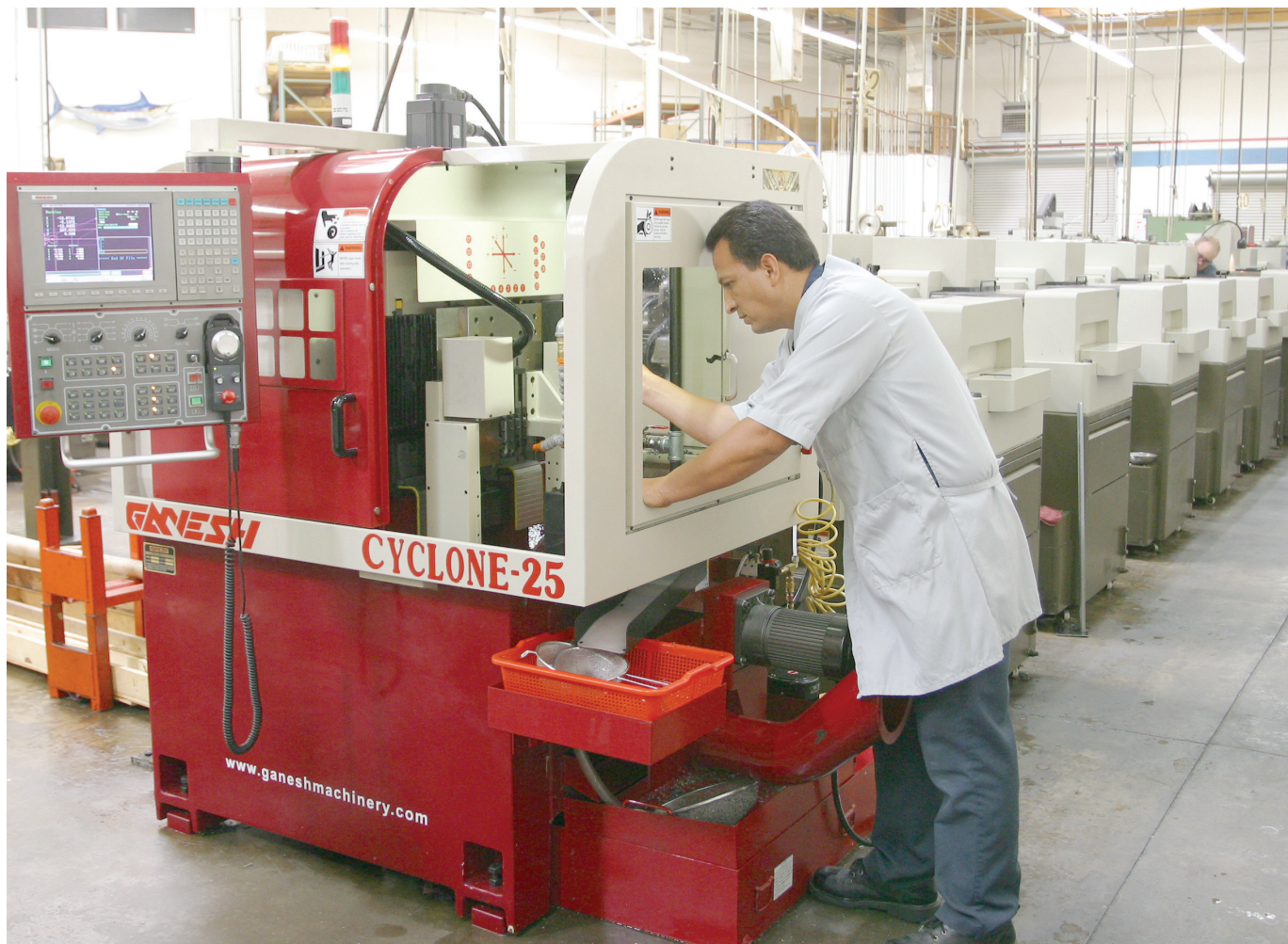
Operator Jose Luis Peredo, Alpha Omega Swiss CNC setup programmer, prepares the company's Ganesh Cyclone-25 multitasking CNC lathe to run titanium orthodontic parts. In the background is a lineup of Citizen machines.
