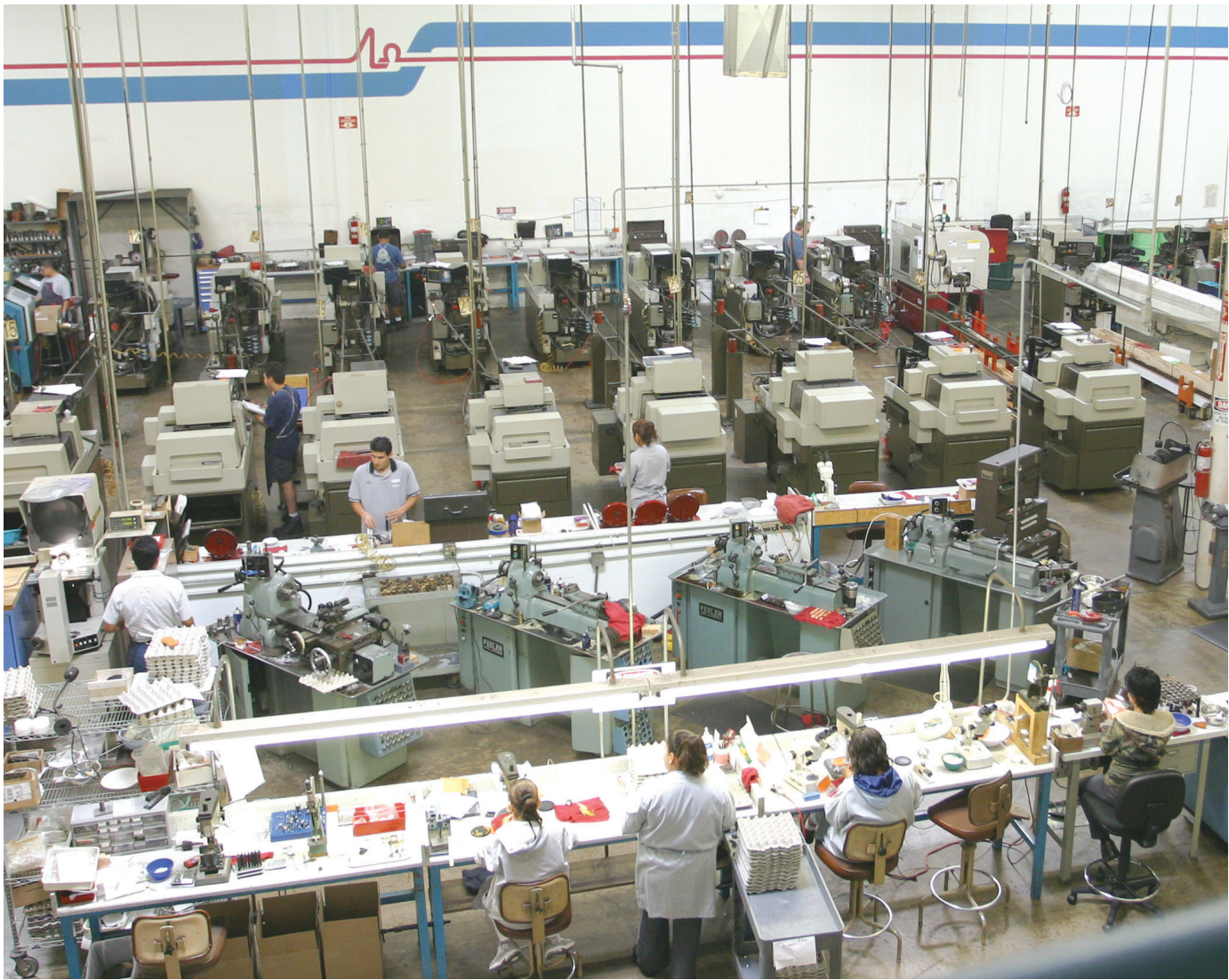
Overview of the Alpha Omega shop floor where the company runs 16 Citizen screw machines, 9 Nakamura lathes, 1 Ganesh Cyclone-25 (upper right-hand corner) and a variety of other machines. The company has 32 employees working in a 16,000 sq ft facility. It's customer list numbers nearly 400 companies.
