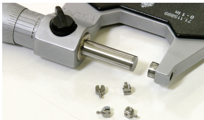
Typical small parts produced by AOS, include these titanium mounts for overbite headgear, made from 1/4” bar stock
