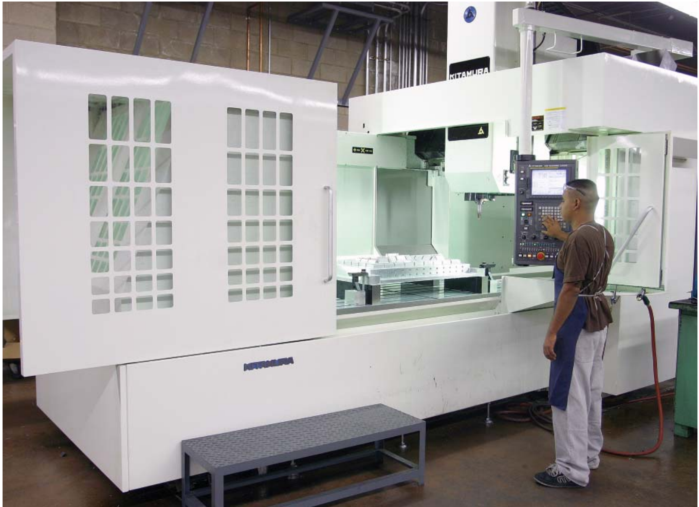
Journeyman mold maker, Ed Espino prepares High Desert's Kitamura Bridgecenter 8 to run a 50" X 35" mold for molding concrete back panels for walls. The Kitamura has a 35.4" x 98.4" table size, 80.0" x 42.7" x 28.0" travel, 40-taper, 20,000 rpm spindle and 80-tool ATC.
