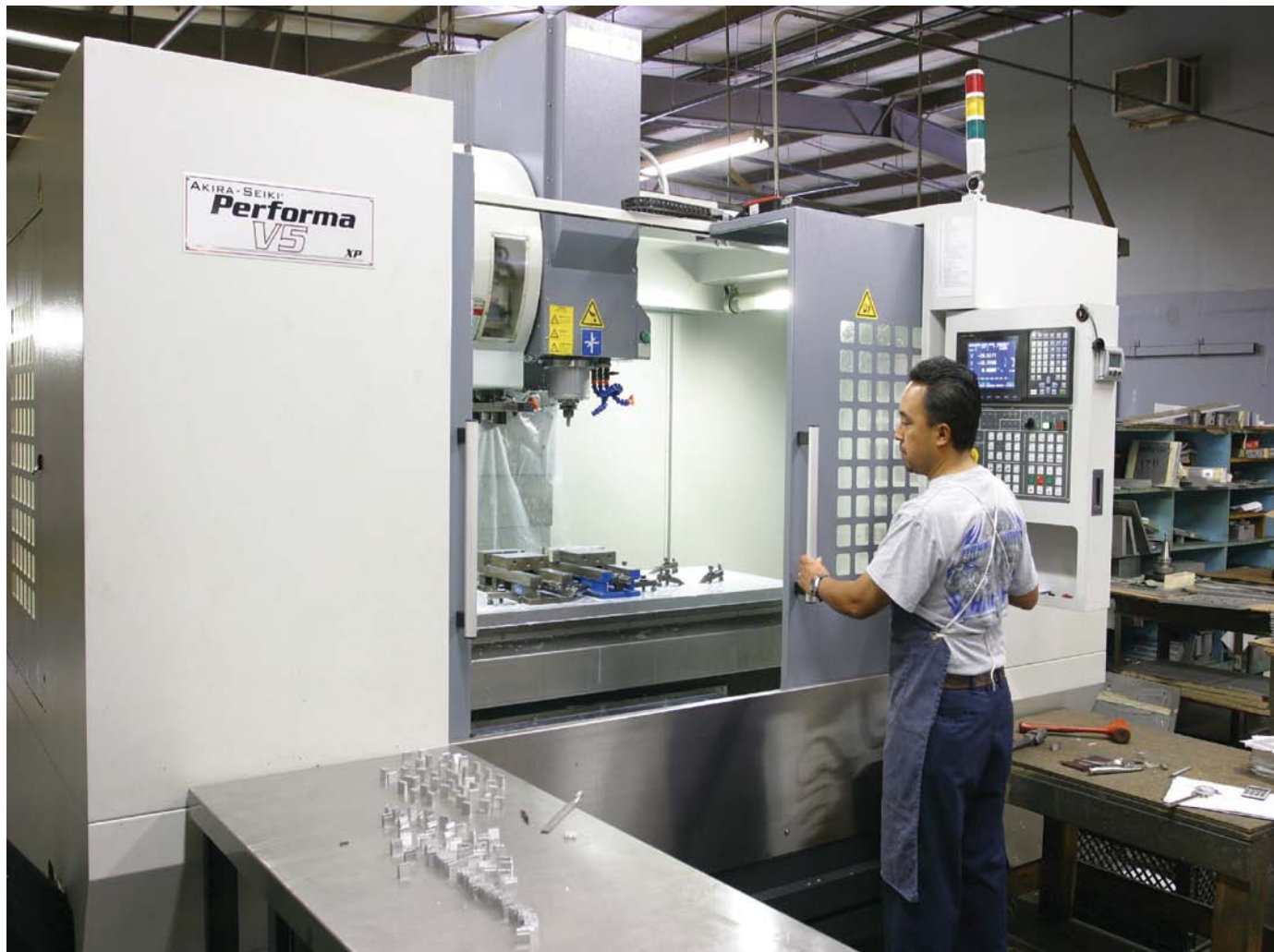
CNC operator Aaron Pachego sets up an Akira Seiki Performa V5 VMC to run chassis hardware.
