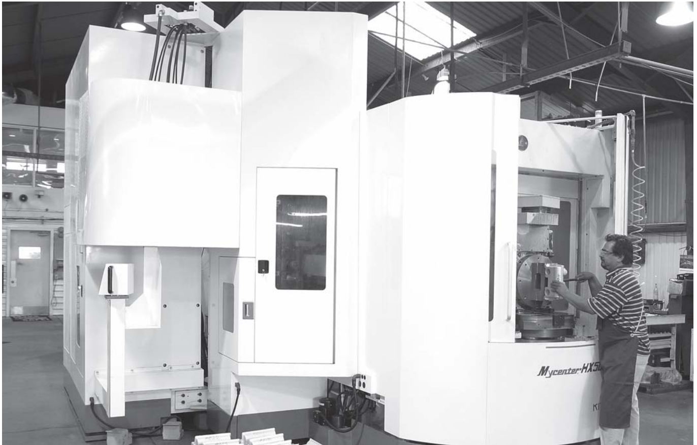
CNC operator, Mario Rivera, loads a part onto a Mycenter HX500i pallet.
