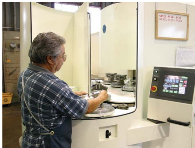
CNC operator Elisio Salgado loads a pallet at the Supercell load station
