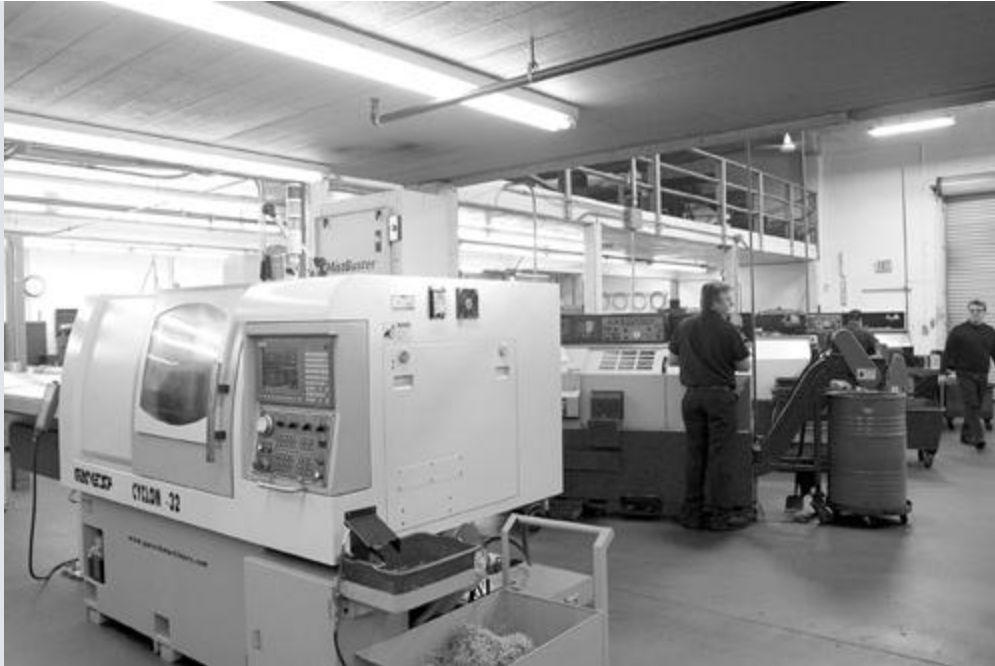
Line up of machines at Heather Screw Products. in the foreground is the Ganesh Cyclone 32, with live tooling and bar feeder. In the background are three Femco Durga 25E lathes. CNC lathe operator is Rafael Vargas.
