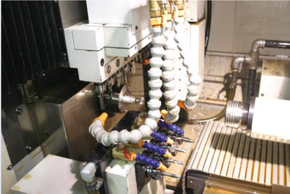
The Ganesh Cyclone GT-32 is a 3-axis 1.25" (32mm) bar diameter gang-tooled CNC screw machine. The gang tool slide allows great flexibility in tool placement. Dual insert boring bars provide two tools in one tool shank. A bank of 4-driven tools can be mounted on the cross slide to work in conjunction with the full C-axis spindle to complete the milling and drilling features on the workpiece. An 8-station tool turret can also be added to the cross slide for additional tooling.
