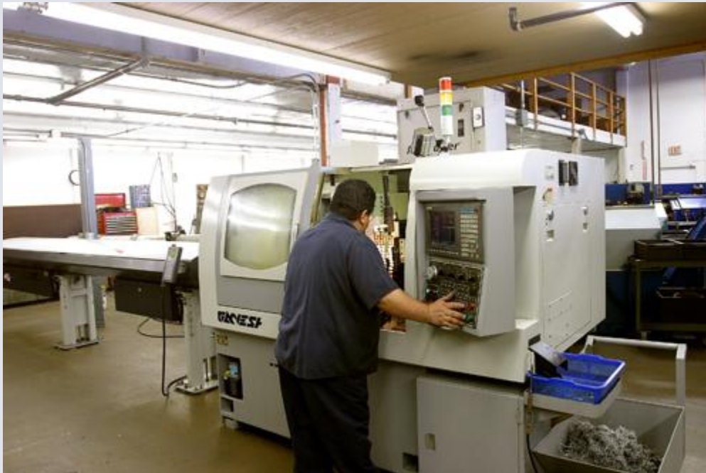
CNC lathe operator Carlos Sandoval sets up the Ganesh Cyclone-32 CS 7-axis twin-spindle CNC turn-mill center with 11 live tools and 27 total tools. The Ganesh is the workhorse for Heather, bringing in business from other shops without multi-axis capability
