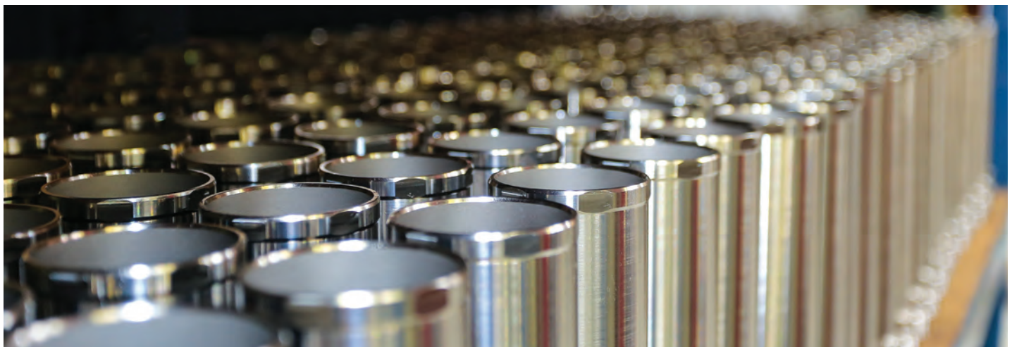
It is no surprise that a company based in Huntington Beach, CA has a thing for tubes. Transfer tubes were a big break for the company 15 years ago and now is one of their most mass produced parts. Transfer tubes are part of the mechanism that controls the flaps on a plane. A 737 uses eight of them per plane.
